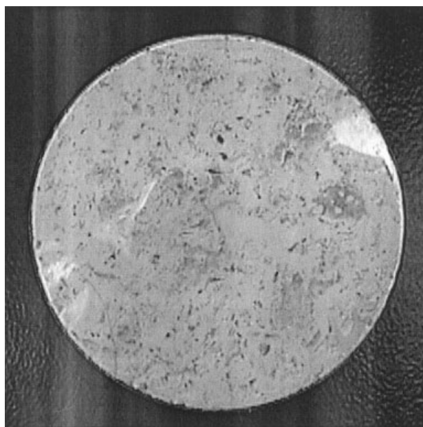
Figure 4 Photograph of a cotton–clay nanocomposite. The nanocomposite sample depicted had a diameter of 4 in.
